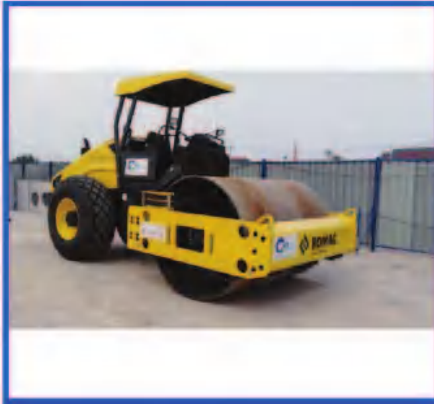
Vibrator Roller 2 units
